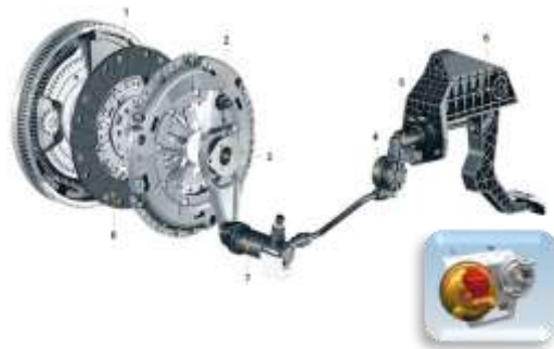
Lower Pedal Effort on Clutch Low Hysteresis clutch along with high size clutch booster Reduced effort by 40% over BS4
